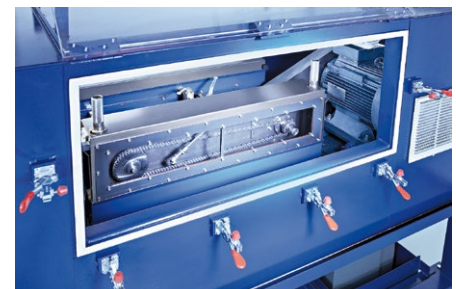
Testing of chain wear elongation behavior on more than 20 test rigs
